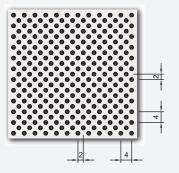
Microperforation Rd 1522 Ø: 1.5mm Open area: 22%
